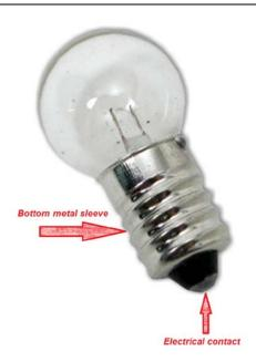
• The "hole of the clothes peg will be lined with the tin foil that makes a path to your conductivity test leads. The electrical contact on the base of the light bulb will then firmly rest on the other strip of tin foil that connects the clothes peg to the battery.
